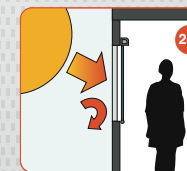
With an interior solar protection system
